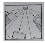
Ultrasonic sound-waves travel in straight lines like audible sounds, echoing off non- absorbing materials. Sound absorbing materials such as carpets, drapes and soft furniture will reduce the range. "Shadow" areas may occur around corners or in nooks and crannies where the sound waves can not reach.
